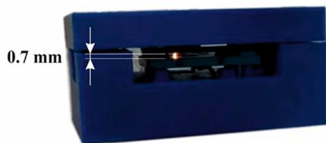
cathode aperture diameter, a He flow rate of 5 L/min, a peak-to-peak voltage of 7.5 kV, a mean current of 4 mA and a frequency of carrier wave of 1.37 kHz. The current value confirmed that it was the glow discharge (Roth et al., 2005). The voltage waveform during the AC-driven discharge are presented in Figure 7.
