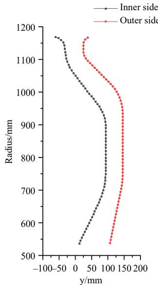
**Figure 2.** Cross-sectional node coordinates of track wheel web
