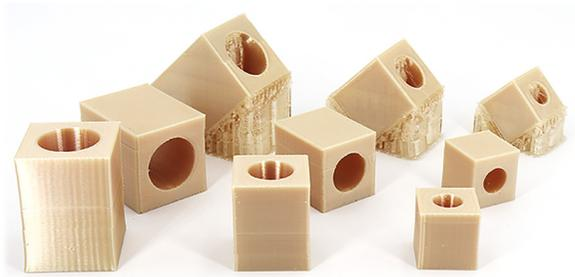
Figure 2 Specimens with machined holes
