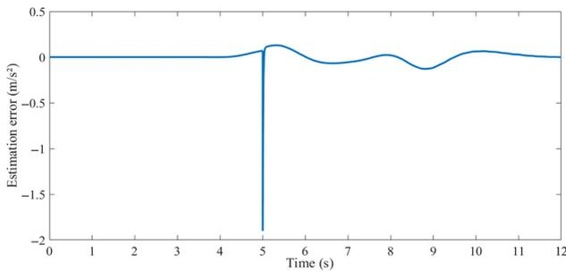
**Figure 20** Fault estimation curve of the rotation angle sensor
