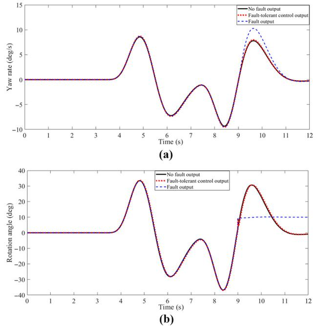
Notes: (a) Performance comparison of the yaw rate sensor before and after fault tolerance; (b) performance comparison of the rotation angle sensor before and after fault tolerance
