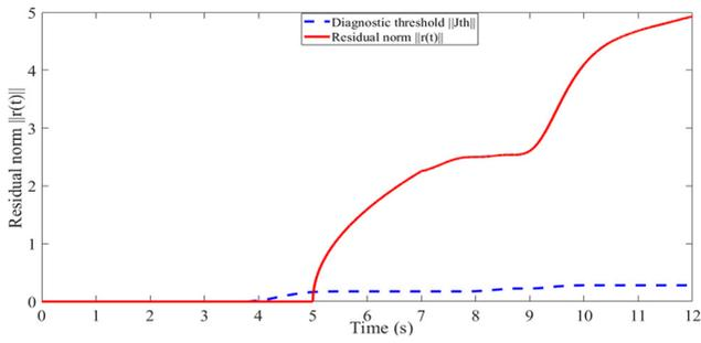
**Figure 10** Results of simultaneous gain-stuck detection of two sensors
