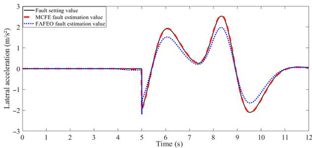
**Figure 19** Fault estimation error curve of the lateral acceleration sensor by estimation method in this paper
