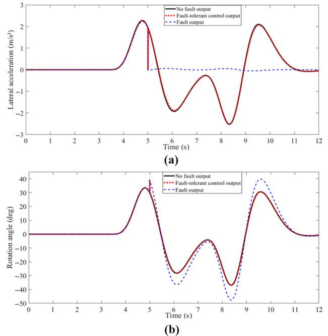
Notes: (a) Performance comparison of the lateral acceleration sensor before and after fault tolerance; (b) performance comparison of the rotation angle sensor before and after fault tolerance
