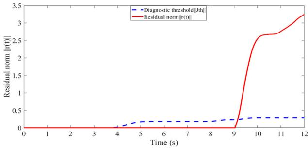
**Figure 11** Results of two sensors interrupted at the same time-gain fault detection
