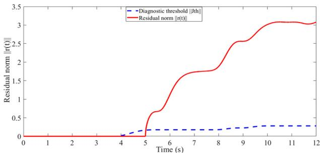
**Figure 12** Fault estimation curve of the rotation angle sensor
