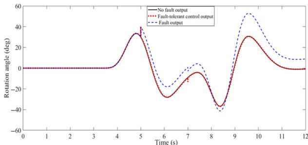
Figure 23 Simultaneous gain-stuck fault tolerant performance before and after comparison curves
