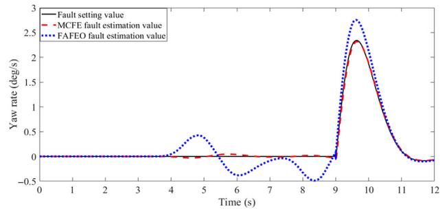
**Figure 15** Fault estimation error curve of the yaw rate sensor by estimation method in this paper
