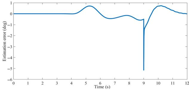
**Figure 18** Fault estimation curve of the lateral acceleration sensor
