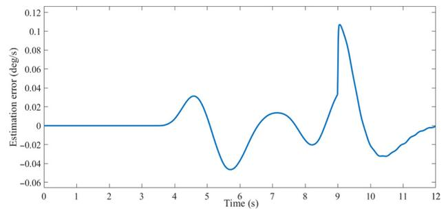
**Figure 16** Fault estimation curve of the rotation angle sensor
