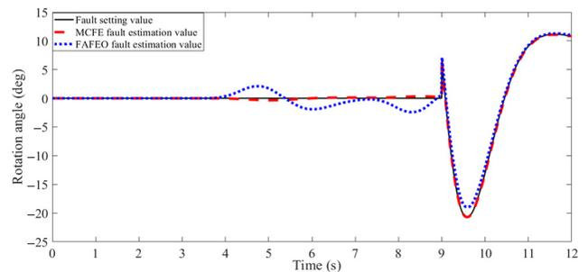
**Figure 17** Fault estimation error curve of the rotation angle sensor by estimation method in this paper
