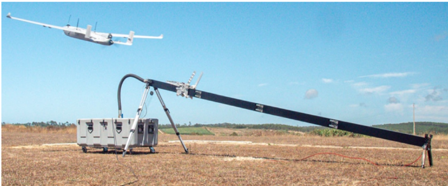
Figure 6. TEKEVER UAV AR3 and other components of UAS
