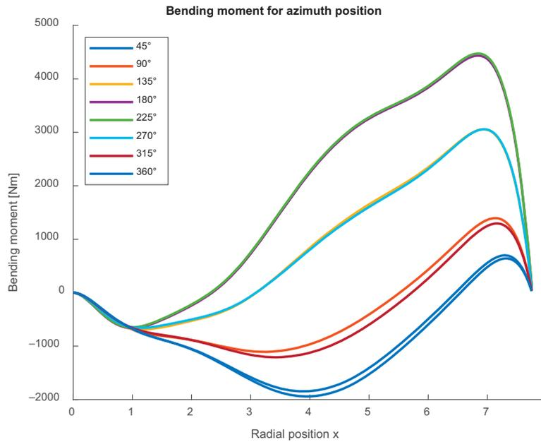
allowing the 3D analysis to provide the total mass of the blade and the mass of the components. The moment acting on a blade in respective sections is loaded from the file generated previously. The strength equations are programmed within the code.
