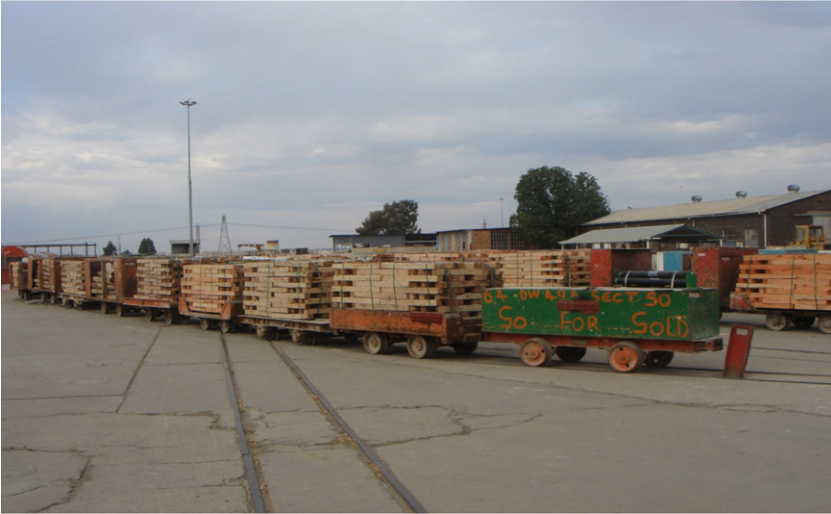
Figure A3: Production Material (Timber Packs, Props, Pipes) Being Transported from Surface to Underground
