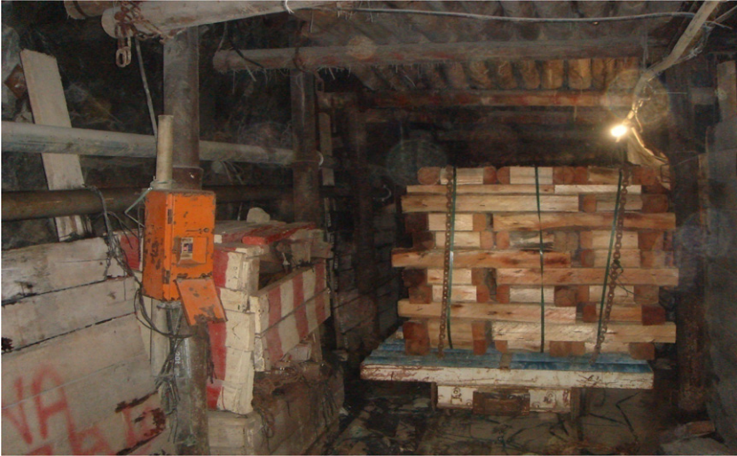
Figure A13: Timber Packs in the Haulage, Underground
