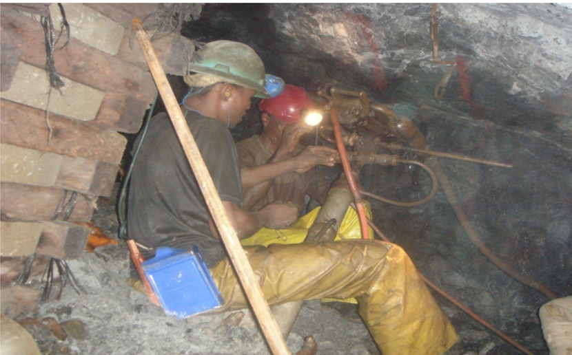
Figure A8: Rock-Drill Operators Drilling the Gold-Bearing Rock (the Reef) by Means of a Pneumatic Drill
