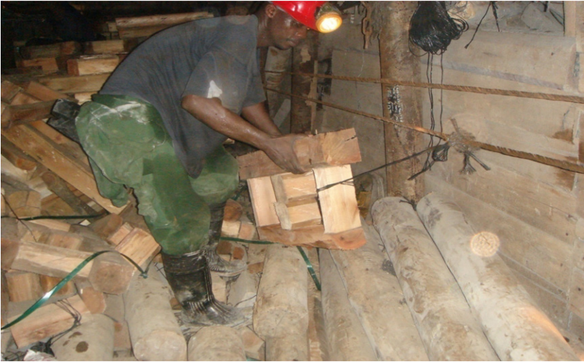
Figure A17: A Team Worker Tying the Timber Pack to the Mono-Winch with a String
